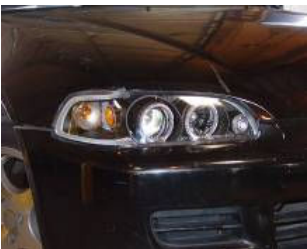
Step 18: Now plug in the new conversion wire harness into the new Anzo head light.
