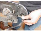
Step 5: Remove the parking light socket from the headlight.
