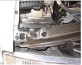
Step 2: Remove the two clips which hold the headlight to the frame.
