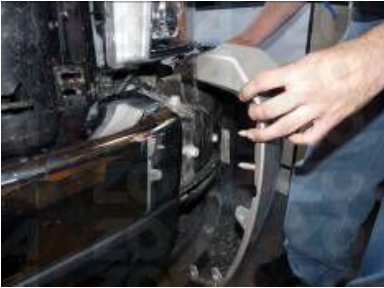
Step 12: Pull off the bumper cover from the frame of the vehicle.
