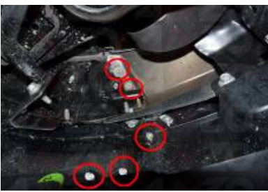
Step 9: Get under the vehicle under the bumper cover to remove the five 10mm screws.
