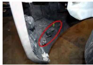
Step 11: Unclip the three pins holding in the bumper cover and the lip.
