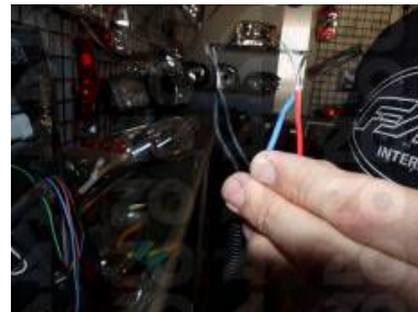
Step 19: Twist the red and blue wires together and the two blacks together from the new headlight.
