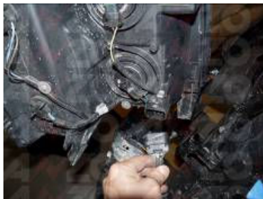
Step 13: Remove the two 10mm screws holding the headlight in place.
