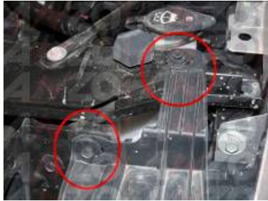
Step 13: Remove the two 10mm screws holding the headlight in place.
