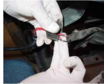
Step 17: Splice the two red wires (1 power; 1 ground) into the parking corner light for the
