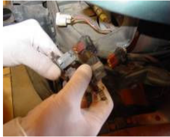
Step 16: Remove the corner light bulbs from the harness.
