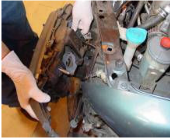
Step 15: Remove the headlight harness and take off the headlight.
