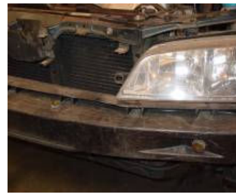
Step 14: Remove the 5/16 hex screw to take off the bumper reinforcement bar.
