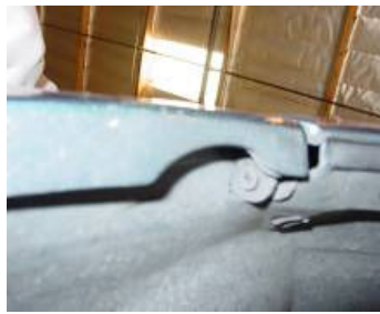
Step 13: Remove the screw on the inside wheel well to take off the bumper.
