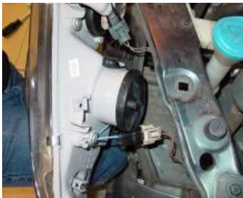
Step 18: Plug in the head light wire harness.
