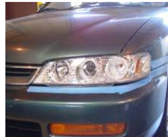
Step 20: Bolt the headlight on and reassemble the bumper back on.
