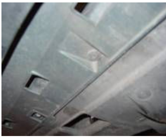
Step 12: Remove the four screws underneath the bumper.
