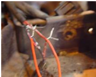
Step 16: Splice the two red wires from the new headlight to the black and red wire to power the halos.
