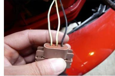
Pictured above is a corner light bulb harness with integrated turn signal and parking light function.
