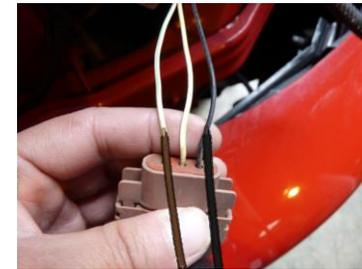
Locate the brown (+) positive wire from the AnzoUSA headlight and splice that wire into the (+) positive turn signal bulb wire. The positive turn signal bulb wire is typically the outside wire opposite of the negative wire.
