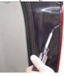
Step 4: Unscrew the two screws with the phillips screwdriver.
