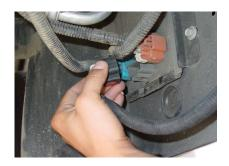
Step 2: Unplug the middle wire harness from the circuit board.
