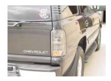
Step 8: Put the tail light in and screw in the two screws to hold the tail light in place.
