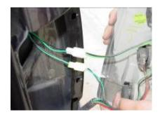
Step 7: plug the two resisters into the tail light.
