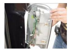
Step 5: Remove the tail light from the vehicle.
