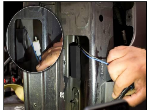
Peel 3m tape backing from resistor and press resistor securely in fender well.
