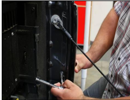
Lower tail gate and remove two 8mm bolts.
