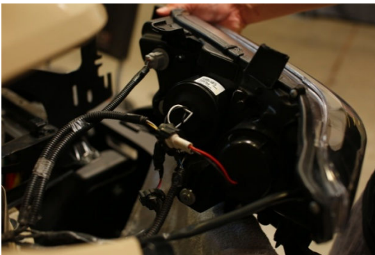
Step 14: Connect all connections into new Anzo headlight (Repeat process on other side)
