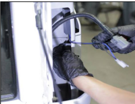
Remove 3m backing tape from resistors and press into fender well securely.
