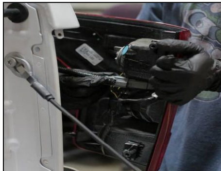
Disconnect main connector harness from factory tail light.
