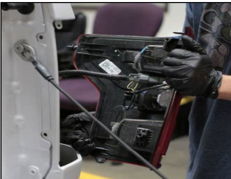
Pull tail light backwards from fender well to remove.
