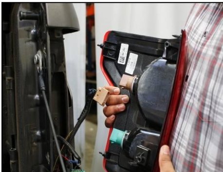
Disconnect both connections from factory tail light.
