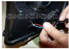
Step 11: Locate the two sets of loose wires from the new Anzo light and twist red with blue.
