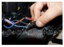
Step 14: Now splice the two black wires into the black wire (-).
