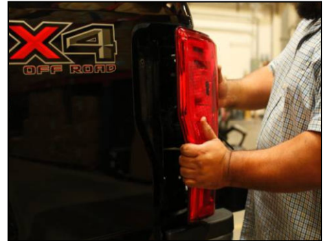
To remove tail light pull light towards side of vehicle to release locating guide pins.
