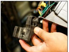
Separate lower headlight mount from factory headlight and set aside.
