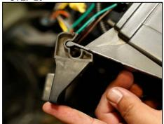
Transfer factory headlight bracket mount to Anzo USA headlight.
