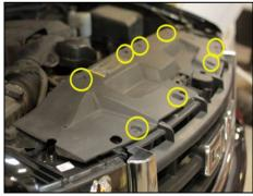
Use panel popper to remove 8 body panel clips on radiator shroud.
