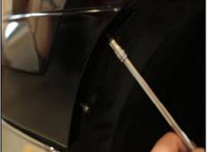
Remove two 7mm bolts on driver's side fender well. Repeat on opposite side.
