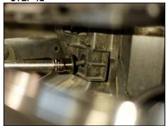
Remove lower 10mm headlight bolt under headlight.
