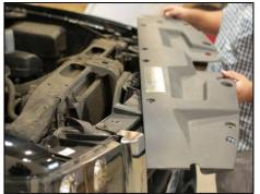
Remove factory radiator shroud and set aside.
