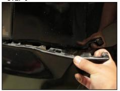
Pull front fascia outward and forward to unclip from fender. Repeat on opposite side.
