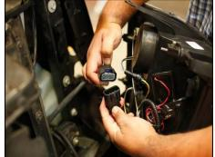
Disconnect main wiring harness from factory headlight.
