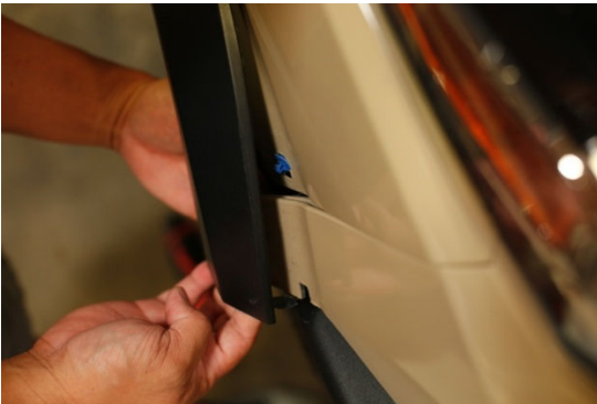
Step 8: Gently pop out fender trim from bumper (Repeat process on other side)
