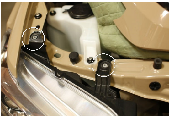
Step 10: Remove two top 10mm bolts from headlight (Repeat process on other side)
