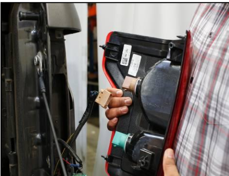
Disconnect both connections from factory tail light.
