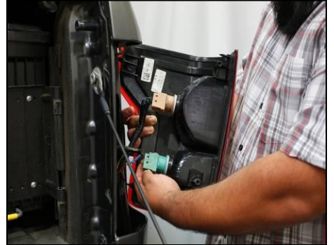
Hold tail light secure in hand and pull tail light towards back of vehicle to remove.
