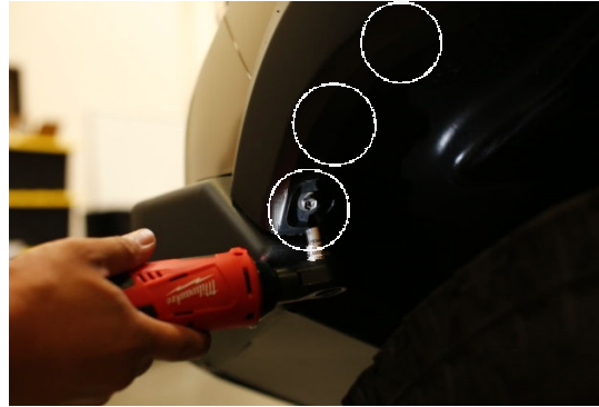
Step 7: Remove 10mm bolt and two plastic tabs from fender inner (Repeat process on other side)
