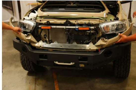
Step 9: Now remove bumper *Customer's Tacoma has aftermarket bumper, you will have to loosen the 8 bolts located under the bumper*
